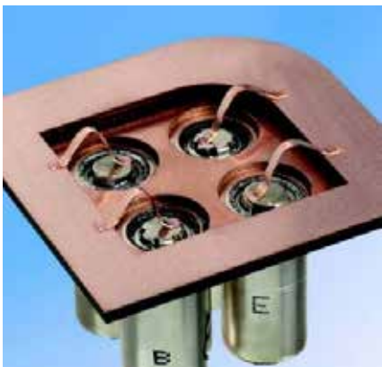
©Fraunhofer ILT: Laser micro welding allows precise and rapid connection of batteries.
