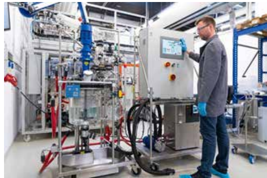
© Fraunhofer IKTS: Holistic recycling solutions on a pilot plant scale for the recovery of battery-grade lithium carbonate (> 99,5 %).
