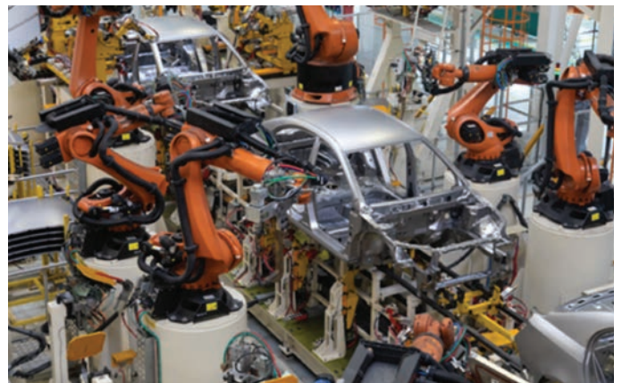
Spot welding (left) in progress on an automotive assembly line (right).
