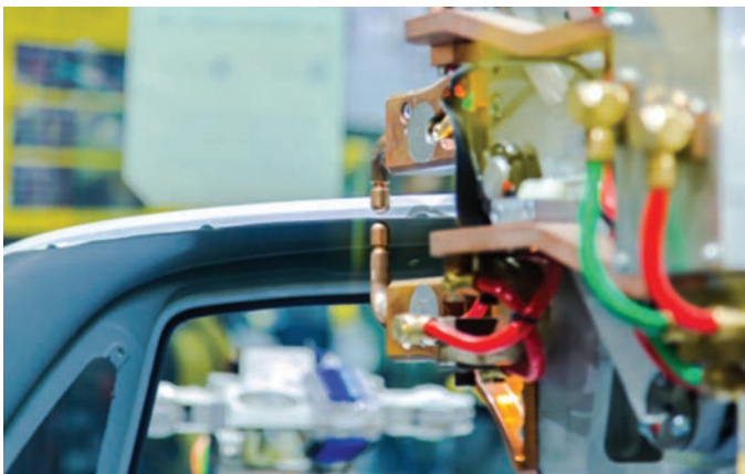
Spot welding (left) in progress on an automotive assembly line (right).
