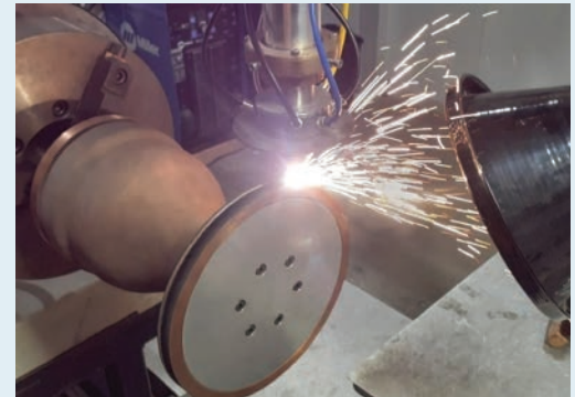
Laser DED process used on NASA combustion chamber
